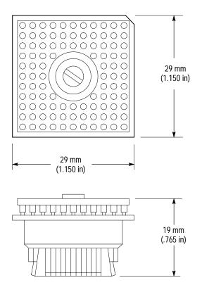
Figure 3–2: Dimensions of the test clip
