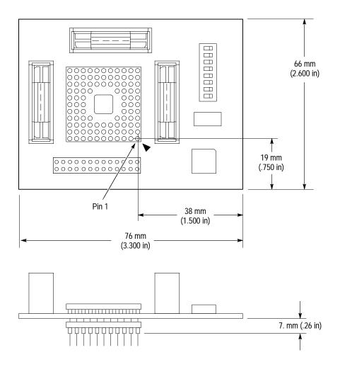
Figure 3–1: Dimensions of the probe adapter
