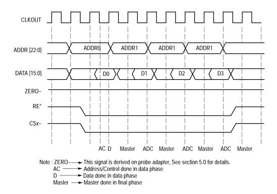
Figure 2-2: MCF5204 Burst cycle bus timing with one wait state
