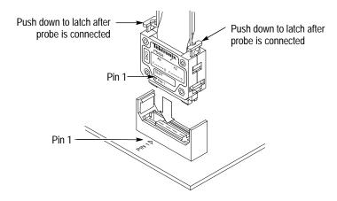
Figure 1–2: Connecting P6434 probes to the probe adapter
