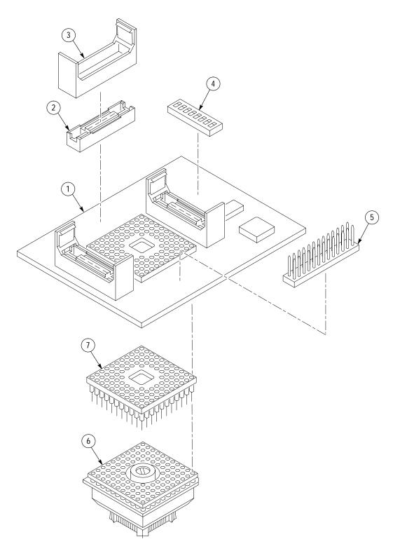
Figure 6–1: MCF5204 probe adapter exploded view
